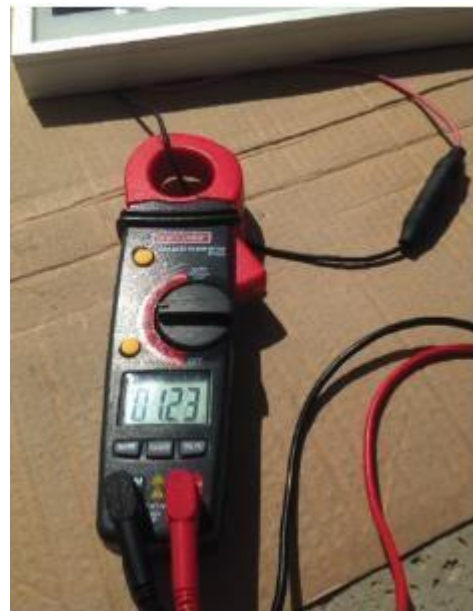
Figure 1.35 : digital clamp-on ammeter with leads is used to perform the circuit measurements.
